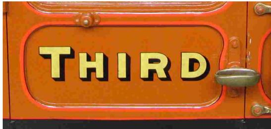
In the case of the sinuate edge of the moulding adjacent passenger door handles, the lining follows the moulding edge, as per above photo.
