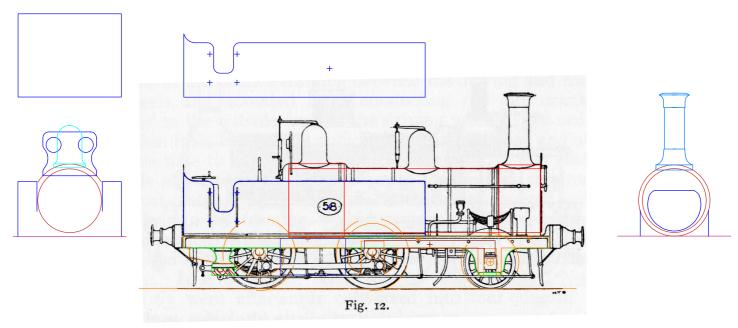
Boiler 4'3" with cladding; Use available 4'6" drivers (lower axle 1.5"); Use available 3'6" trailing (raise axle 1"); Centre wheel moved forward 0.5"; Make coupling rods 7'6" (not true 7'5.5"); use spare 175 rods Brake hangers adjusted to suit spares from 167 2 stage drive to rear wheel [London Rd. box]
